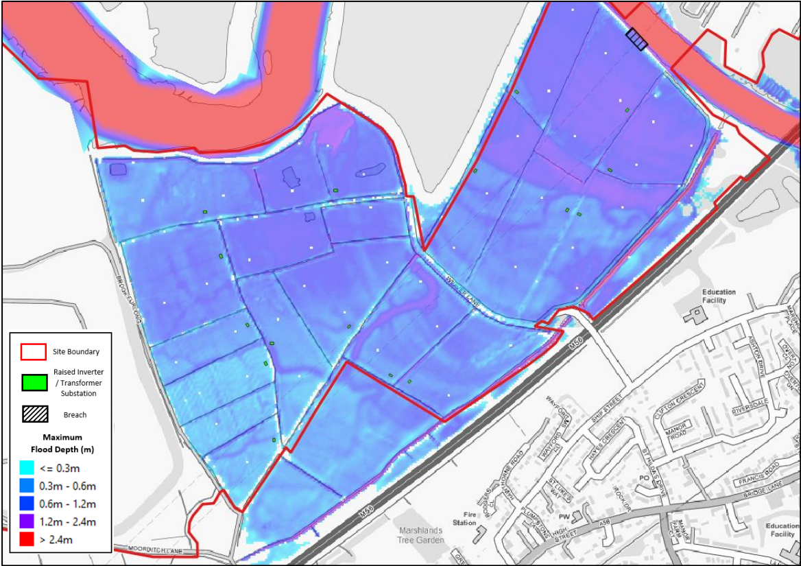
River Weaver Breach 2 1% AEP plus 67% Climate Change Event – Time of Inundation 23hrs
