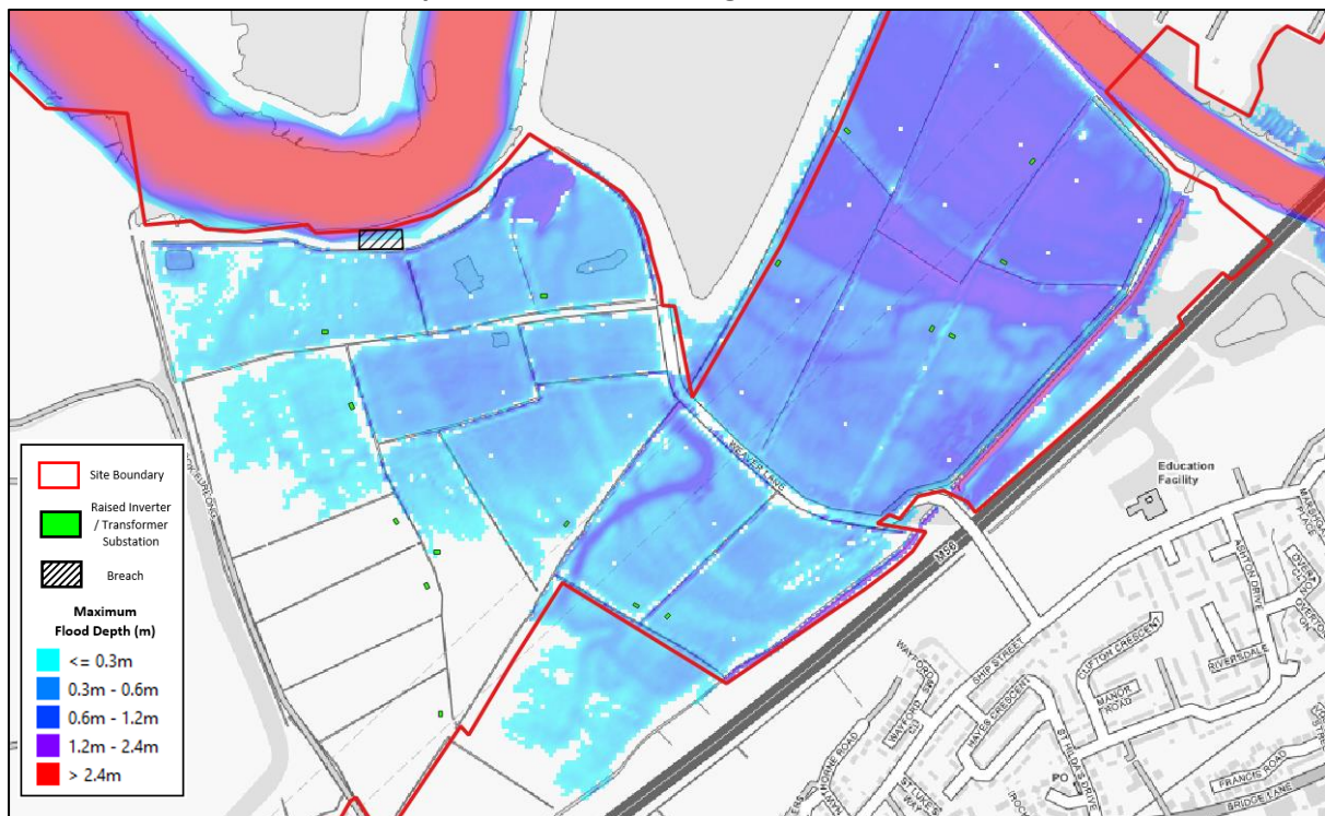
River Weaver Breach 1 1% AEP plus 67% Climate Change Event – Time of Inundation 16hrs
